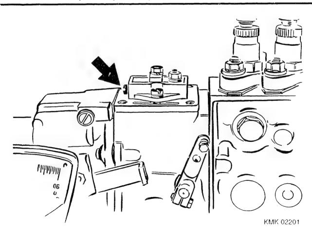
\* Lug cam with torque control
